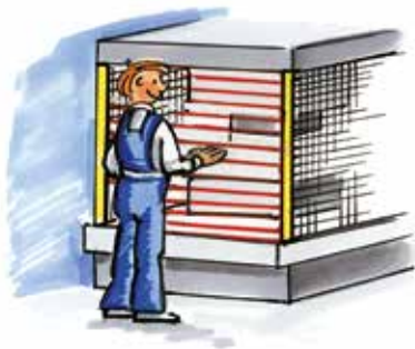
Light curtain for short safe/minimum distances
