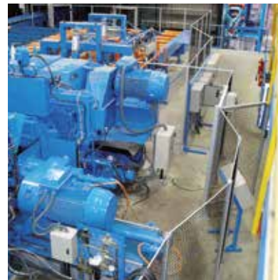
Quick-Guard Express with few components and easy to angle at up to 45°.
