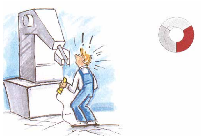
When the three position button is pushed all the way in you will obtain a dual stop. It is essential that the machine stops in an emergency situation.
