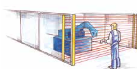
Light curtain for inner area limiting
